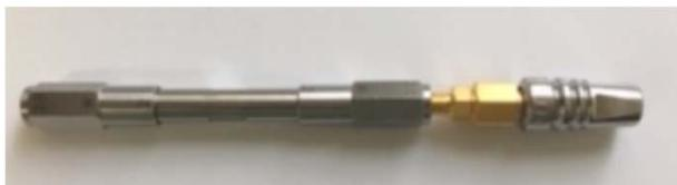
ACQUITY UPLC™ column In-line filter Unit (据え付け時のまま)
