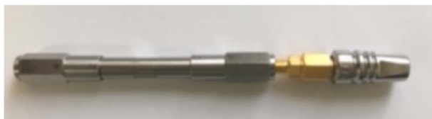
ACQUITY UPLC™ column In-line filter Unit (据え付け時のまま) + Develosil UHPLC C18, 1.6 \mu m
