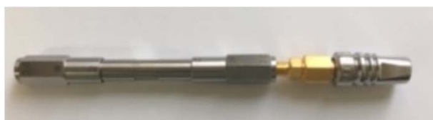
ACQUITY UPLC™ column In-line filter Unit (調整済み) + Develosil UHPLC C18, 1.6 \mu m
